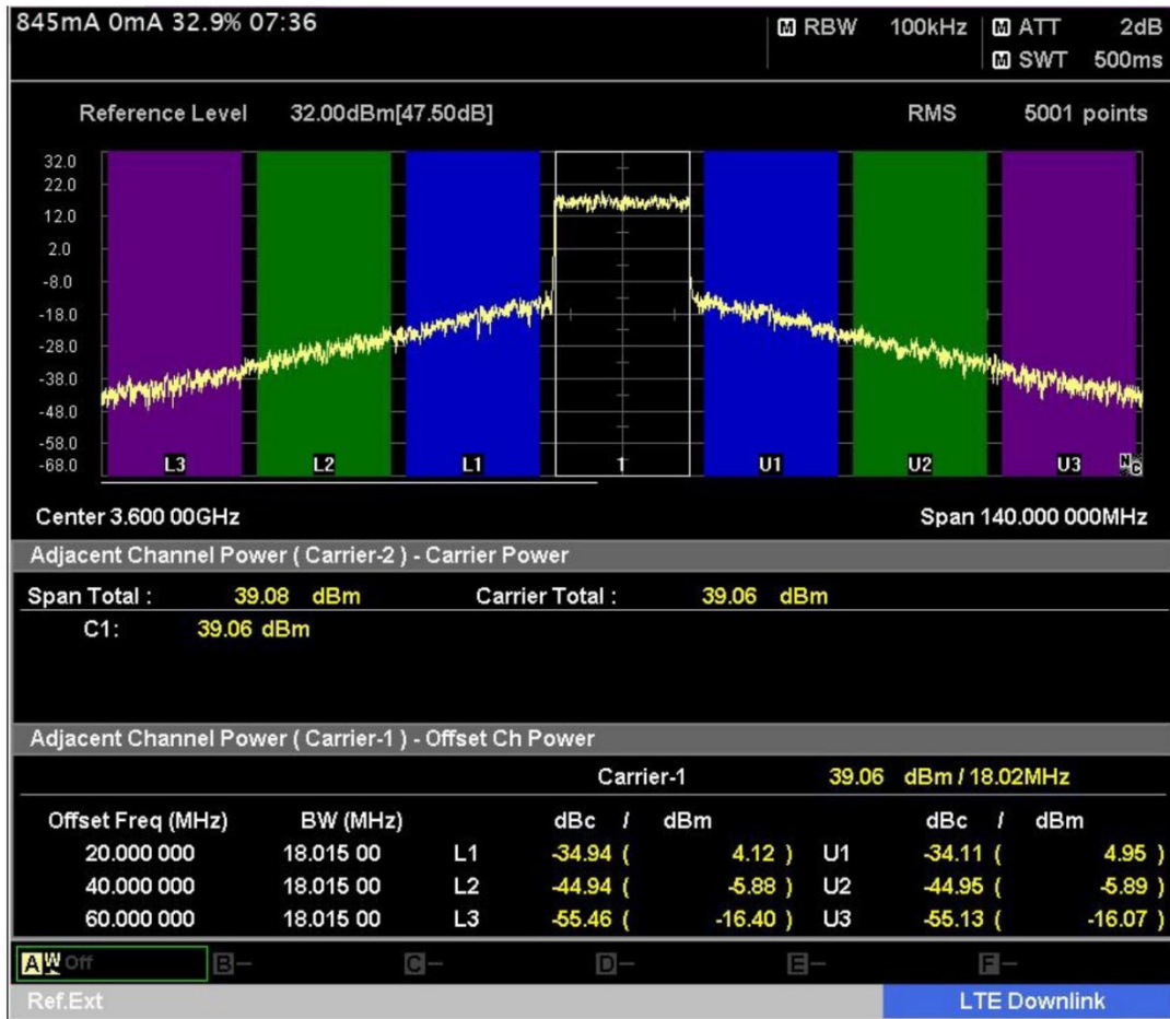
Figure A-1. Output spectrum, uncorrected (20 MHz LTE, 7.5 dB PAR, 200 MHz IBW)
