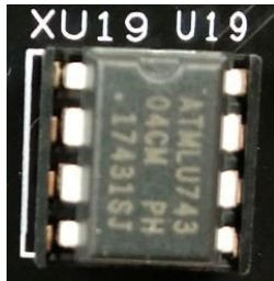
Figure 10. EEPROM in Socket
