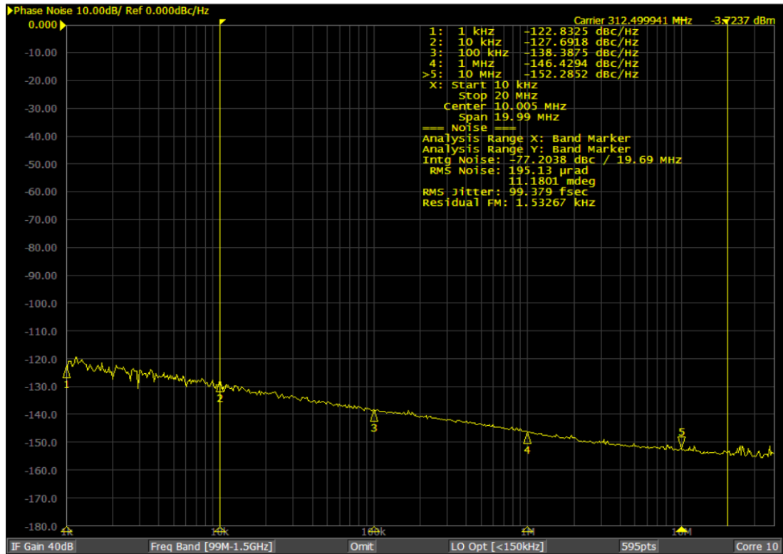
Figure 9. Phase Noise of 312.5MHz Output in Jitter Attenuator Mode
