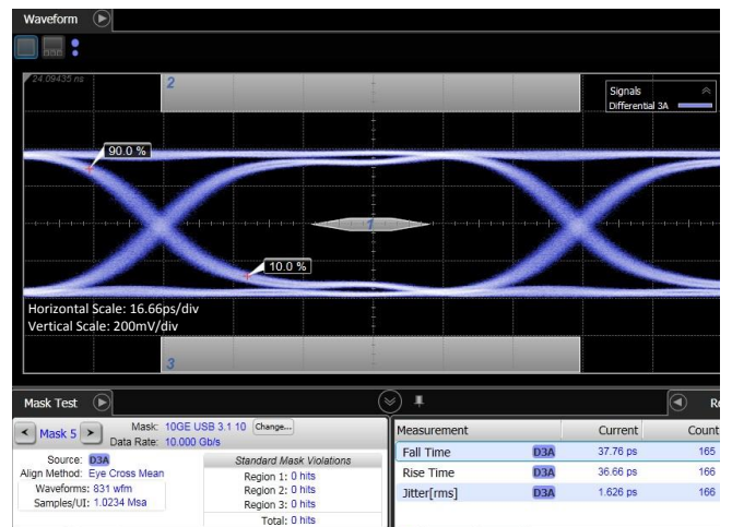
10Gb/s (USB 3.1) Eye Diagram without RClamp3371ZC
