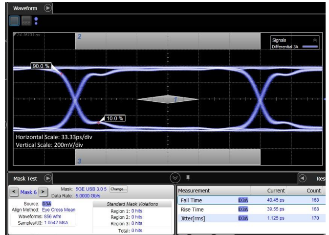
10Gb/s (USB 3.1) Eye Diagram without RClamp3371ZC
