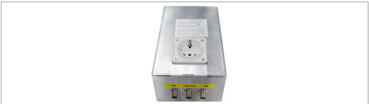
Figure 6: Universal PLC Signal Splitter
