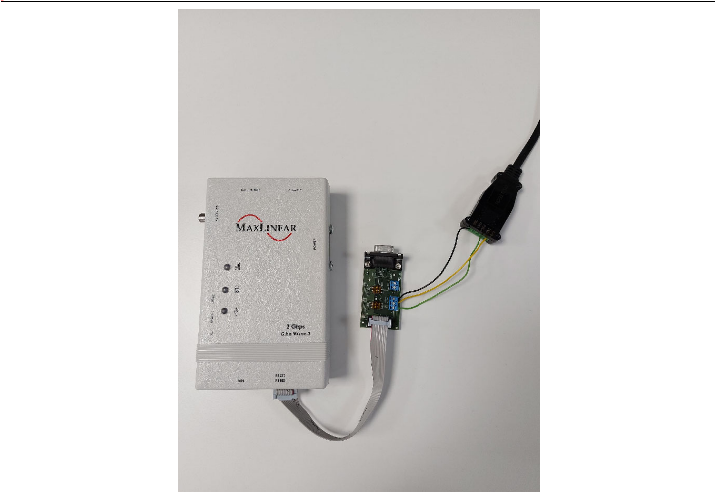
Figure 14: 10pin RS-485 Interface Connected to the USB to the RS485 Cable (Half Duplex)
