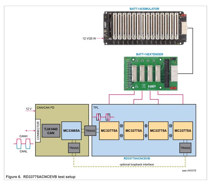
J25 connector can be used to power MC33665A and CAN or CAN FD communication to RD33775ACNCEVB. Electronic control unit (ECU) or CAN tool can be interfaced to J25 for establishing CAN or CAN FD communication.
