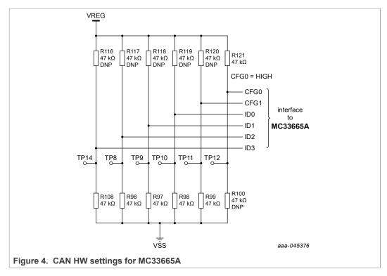
Based on the circuit shown in Figure 4, CFG0 is set to HIGH and CFG1 is set to LOW. CAN communication can be established with 500 kbit/s of baud rate and CAN FD arbitration baud rate is fixed at 500 kbit/s. ID0, ID1, ID2, and ID3 in the CAN ID are set to zero.
