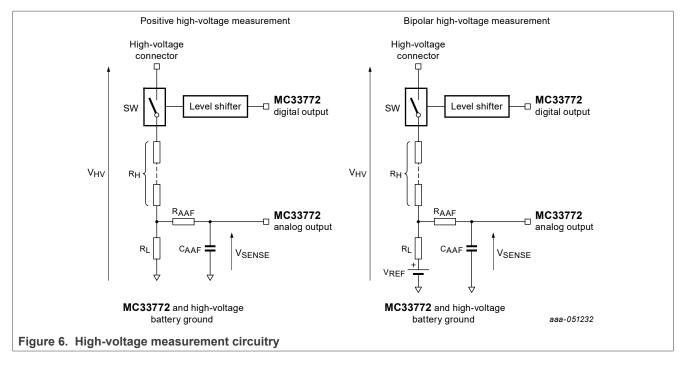
In order to reduce the leakage current in the resistors when there is no measurement, a high-voltage switch can disconnect the bridge. A MC33772C digital output and a level-shifter control this switch.
