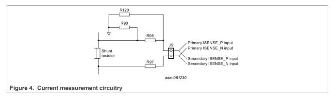
The resistors placement defines whether the two MC33772C measure the voltage drop across the shunt resistor or across the connector, as explained in <u>Table 8</u>.
