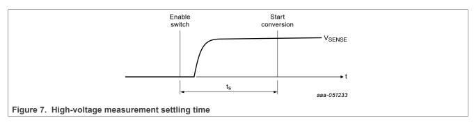
The MC33772C measures the divided voltage. To improve the accuracy, the user should configure the analog input as a single-ended input.
