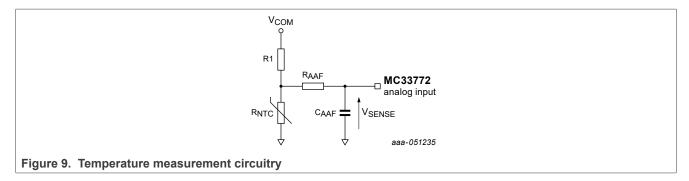
The regulated output voltage of the MC33772C (V<sub>COM</sub>) powers the voltage divider with the NTC resistor. To improve the accuracy of the measurement, the user should configure the analog input as ratiometric input.
