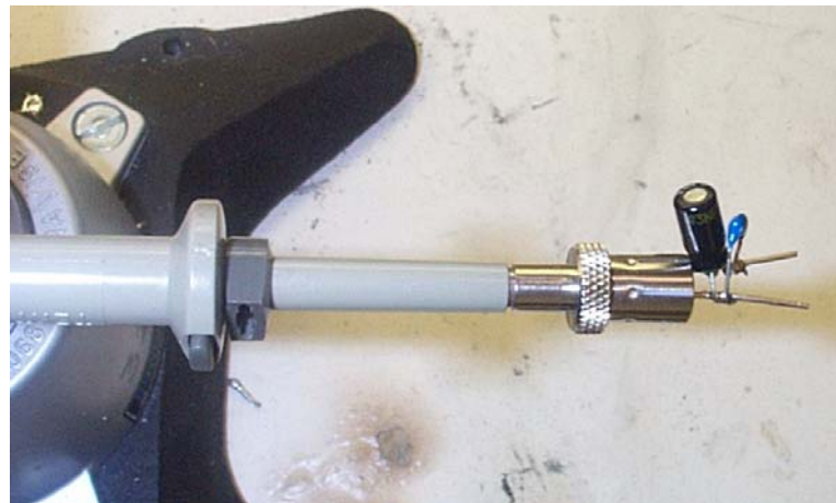
Figure 22 – Oscilloscope Probe with Probe Master ( www.probemaster.com ) 4987A BNC Adapter. (Modified with Wires for Ripple Measurement, and Two Parallel Decoupling Capacitors Added)
