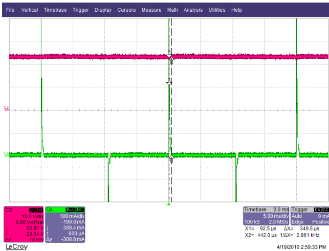
Figure 36 – 230 VAC, 6° Phase. Upper: V_{OUT} , 10 V / div. Lower: I_{IN} , 0.1 A / div., 5 ms / div.
