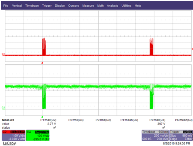
Figure 40 – 265 VAC 60 Hz, Output Short. Upper: I_{DRAIN} , 1 A / div. Lower: V_{DRAIN} , 100 V, 200 ms / div.
