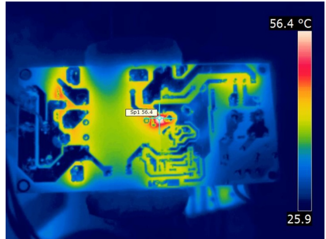
Figure 19 – Blocking Diode D4 (Sp1) Case Temperature.
