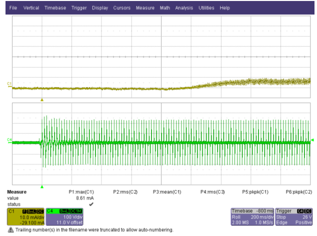
Figure 71 – 120 VAC, 60 Hz. Upper: I_{OUT} , 5 mA / div. Lower: V_{IN} , 100 V, 200 ms / div.
