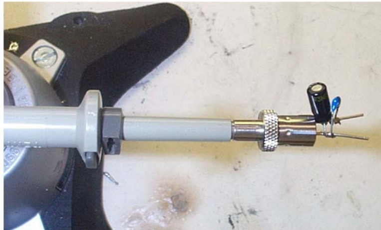
Figure 36 – Oscilloscope Probe with Probe Master ( www.probemaster.com ) 4987A BNC Adapter. (Modified with wires for ripple measurement, and two parallel decoupling capacitors added)
