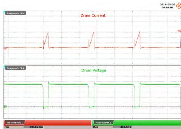
Figure 76 – 300 VAC, 48 V LED Load. Upper: I_{DRAIN} , 100 mA / div. Lower: V_{DRAIN} , 100 V / div., 5 \mu s / div.
