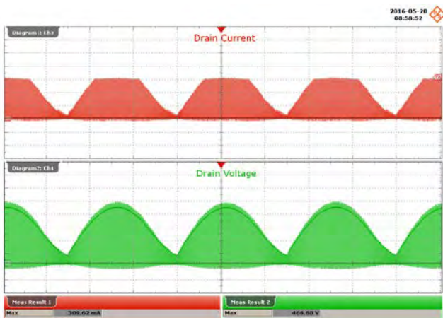
Figure 75 – 300 VAC, 48 V LED Load. Upper: I_{DRAIN} , 100 mA / div. Lower: V_{DRAIN} , 100 V / div., 4 ms / div.
