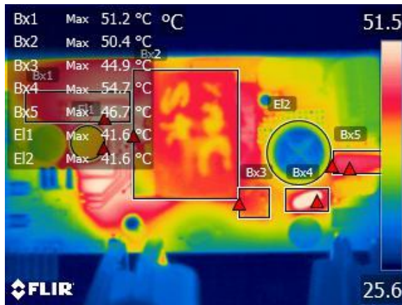
Figure 35 – Top Components, Ambient = 27 °C. Bx1: SR FET, PCB = 51.2 °C. Bx2: Transformer = 50.4 °C. Bx3: Primary Snubber = 44.9 °C. Bx4: Thermistor = 54.7 °C. Bx5: Bridge Diodes = 46.7 °C. E1: Output Capacitor = 41.6 °C. E2: Input Capacitor = 41.6 °C.
