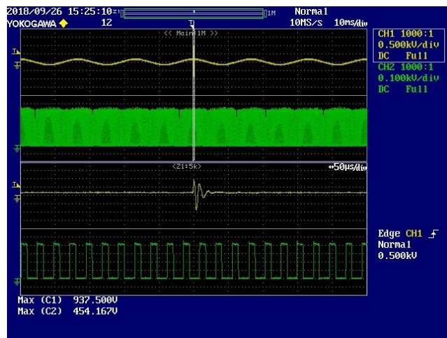
Figure 138 – (+) 2.5 kV Ring Wave Surge, 90° Phase Angle. Lower: V_{DRAIN} , 100 V / div., 10 ms / div. Peak V_{DRAIN} : 454.17 V.
