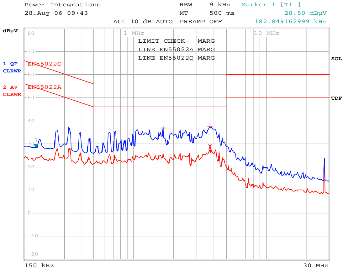
Figure 26 – Conducted EMI, Maximum Steady State Load, 115 VAC, 60 Hz, and EN55022 B Limits.
