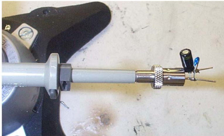
Figure 11 – Oscilloscope Probe with Probe Master ( www.probemaster.com ) 4987A BNC Adapter. (Modified with wires for ripple measurement, and two parallel decoupling capacitors added)
