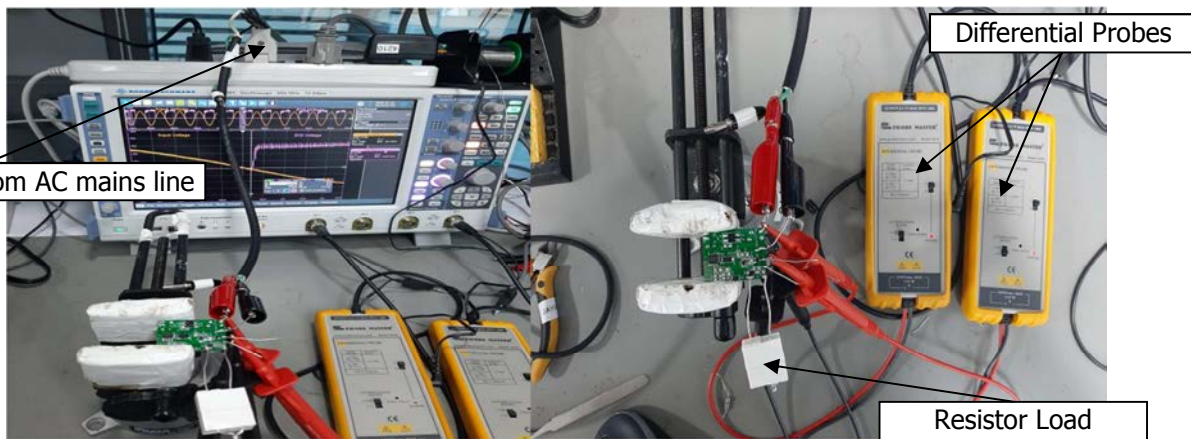
Figure 73 – ZCD Voltage Measurement Set-up.
