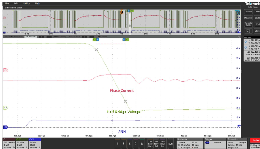
Figure 27 – Drain Voltage (Turn-On) 70 W Inverter Output Power. CH1: I_{PHASE} , 500 mA / div. CH2: V_{HB} , 50 V / div. CH3: V_{INH} , 5 V / div. Time: 2 ms / div. Zoom: 100 ns / div. Turn-On Slew Rate: 2.12 V / ns.
