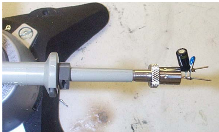
Figure 114 – Oscilloscope Probe with Probe Master ( www.probemaster.com ) 4987A BNC Adapter. (Modified with wires for ripple measurement, and two parallel decoupling capacitors added.)
