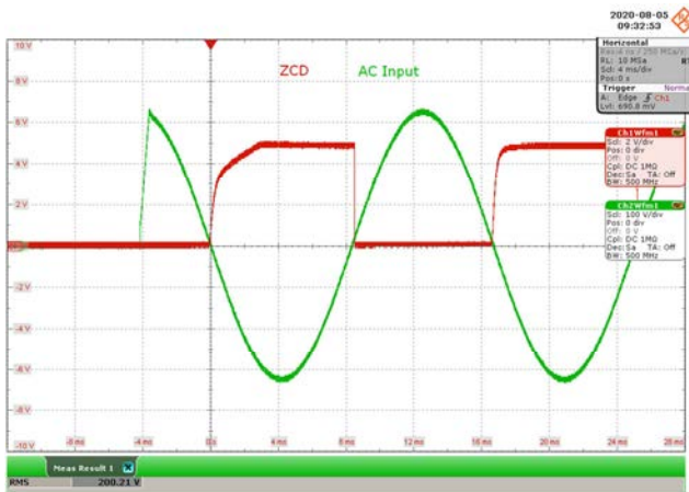
Figure 29 – 230 VAC 50 Hz, No Load CH1: ZCD, 2 V / div., 4 ms / div. CH2: V_{IN} , 100 V / div., 4 ms / div.
