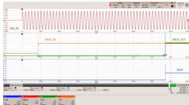
Figure 34 – Input Voltage, Output Voltage and Current. 265 VAC, 5.0 V, 3 A (E-load CC Mode). V_{BUS\_IN} = 5.159 V Steady-State. t_{output\_delay} = 769 ms CH1: I_{OUT} , 1 A / div. CH2: V_{IN\_AC} , 100 V / div. CH3: V_{BUS\_OUT} , 1 V / div. CH4: V_{BUS\_IN} , 1 V / div. Time: 100 ms / div.
