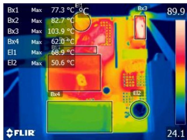
Figure 30 – Top Thermal Image, T_{AMB} = 27.9\text{ }^{\circ}\text{C} .
