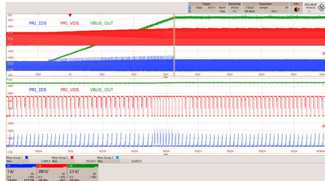
Figure 60 – Primary Drain Voltage and Current. 265 VAC, 3.3 V to 21 V V_{OUT} Transition, 2.85 A Load. V_{DS\_PRI} = 553.36 V Maximum. CH1: I_{DS\_PRI} , 1 A / div. CH2: V_{DS\_PRI} , 200 V / div. CH3: V_{BUS\_OUT} , 2.5 V / div. Time: 20 ms / div. (100 \mu s / div. Zoom).
