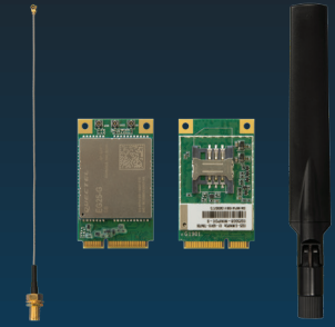
LTE Connectivity mPCIe Quectel 4G LTE CAT4 Global module EG-25G
