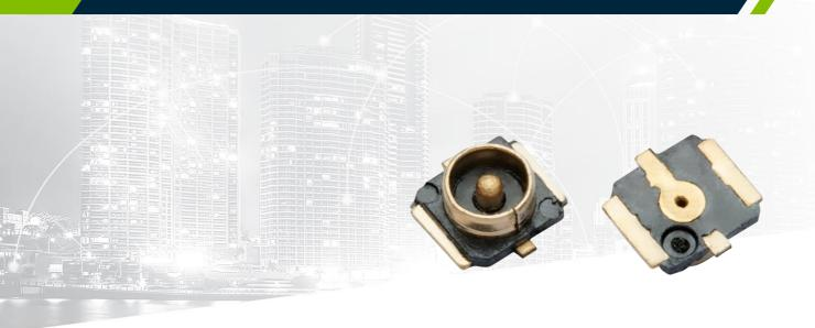
Part of the Taoglas SMD Mount Receptacle the RECE.20369.001E.01 is a 3-pad type wire-to-board SMD Receptacle solution that is ultra-small, lightweight and low profile (1.6mm MAX.) with an operational frequency range of DC to 6 GHz. Taoglas the RECE.20369.001E.01 is gold plated to have superior performance and allow easy mounting of the male RF connector.
