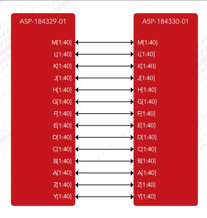
Note: Block diagram shows pin numbers and not signal names
