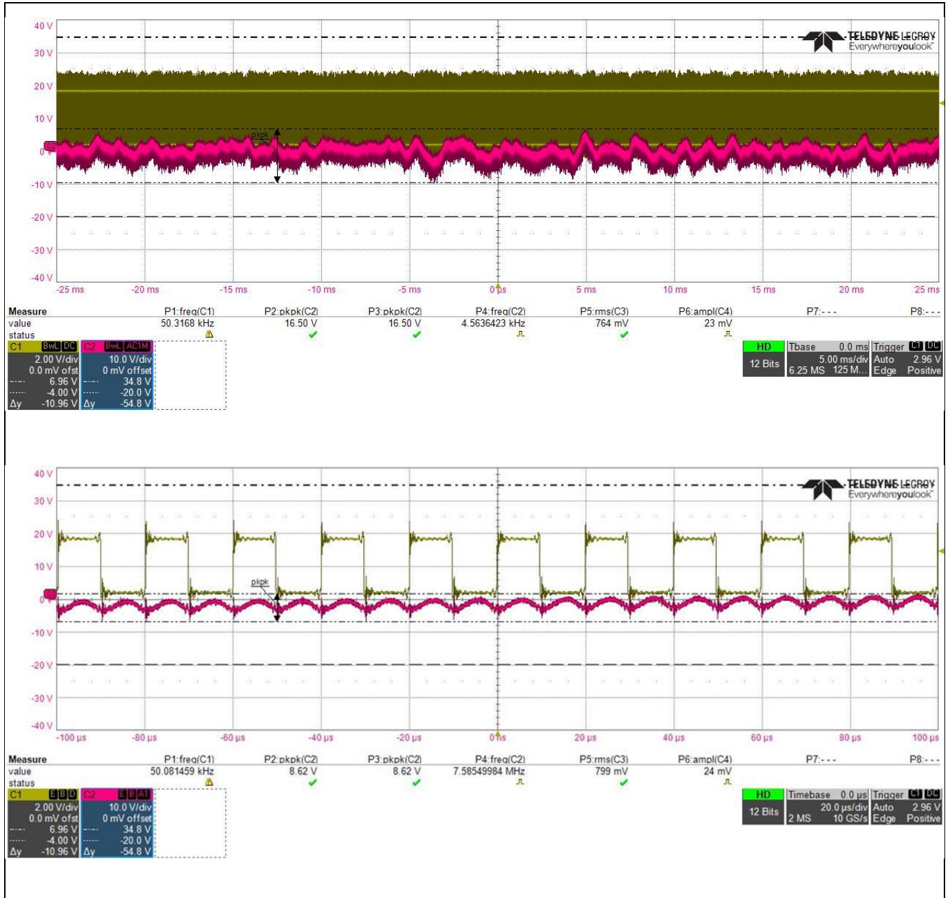
Figure 13 Output voltage ripple
