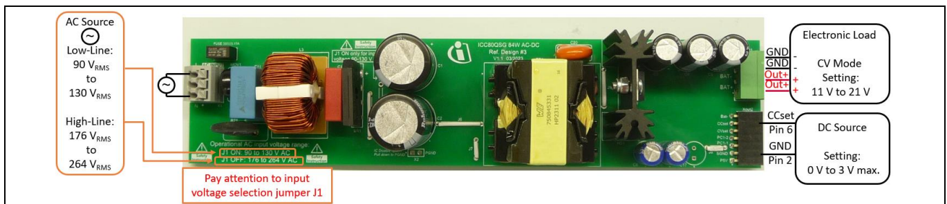
Figure 2 Test setup with electronic load and adjustable CC set-point using DC source
