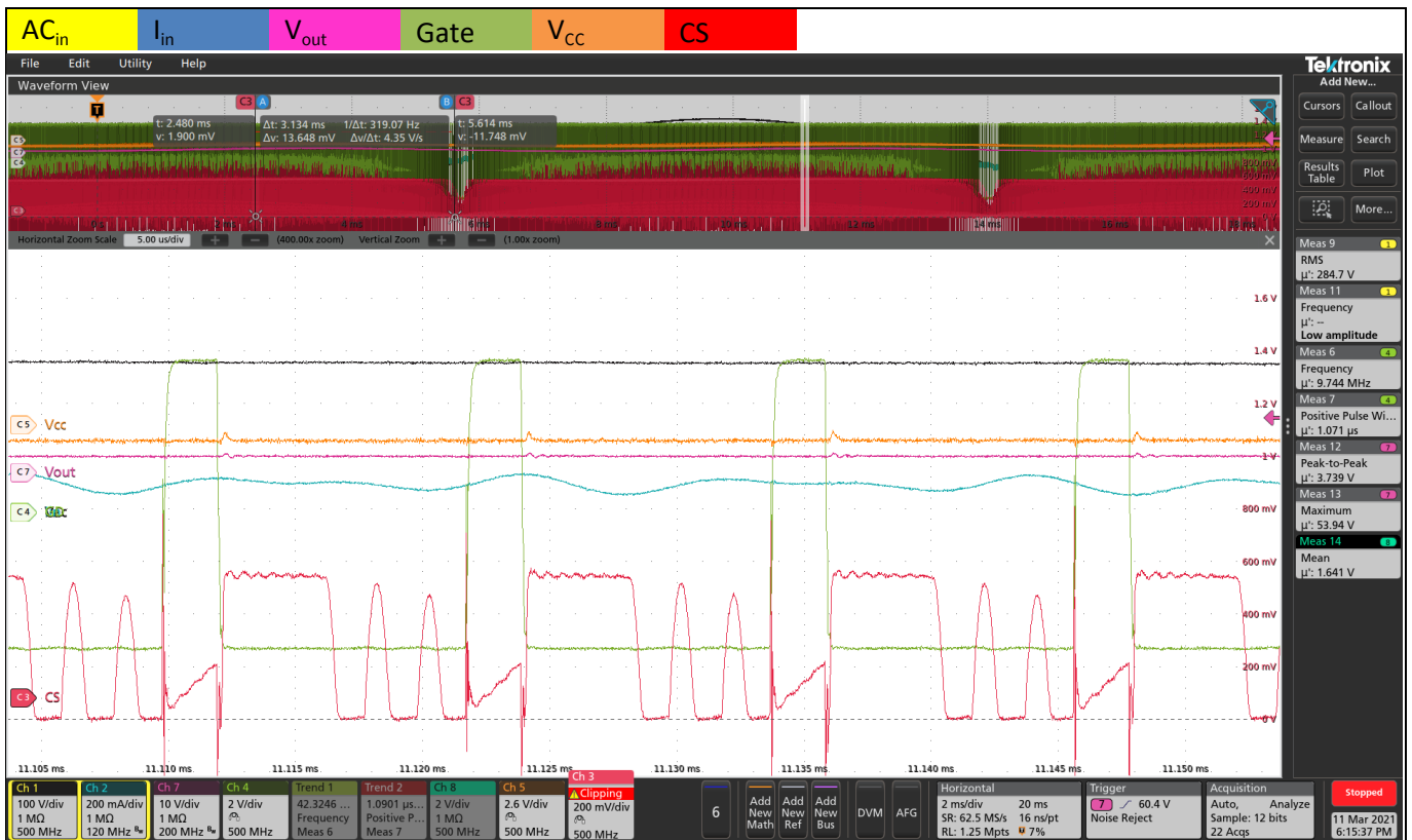
Figure 31 230 V third valley operation ( V_{out} ripple pk-pk 3.7 V)
