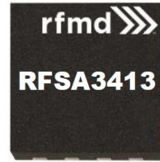
16 Pad 3.0 x 3.0 x 0.85 mm QFN Package
