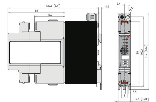
Housing width tolerance +0.5mm, -0mm as per DIN 43880. All other tolerances +/- 0.5mm. Dimensions in mm.
