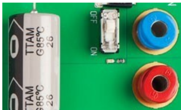
Figure 3.2 One of the two RC switches in “Off” position
