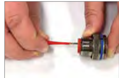
Plastic tool with contact in proper position.
