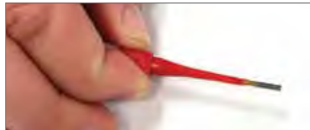
Plastic tool with contact in proper position.
