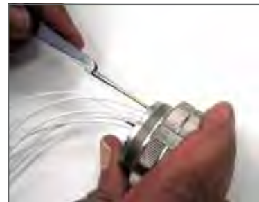
Removal of contacts with metal tool.
