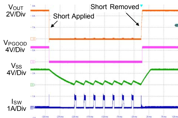
Figure 3. Short Circuit Protection and Recovery
