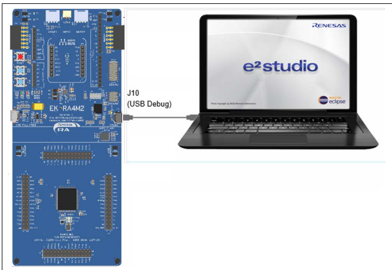
Figure 23. Connecting the EK-RA4M2 Board to the Host PC via USB Debug Port
