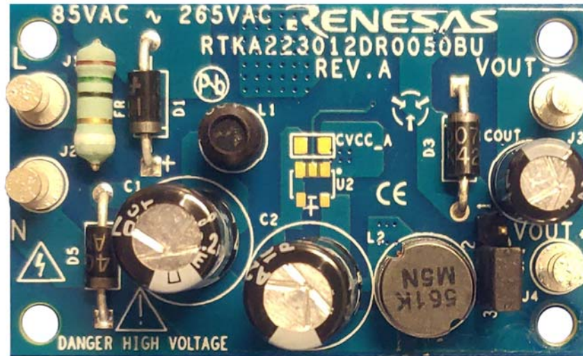
Figure 2. RTKA223012DR0050BU Evaluation Board (Top)
