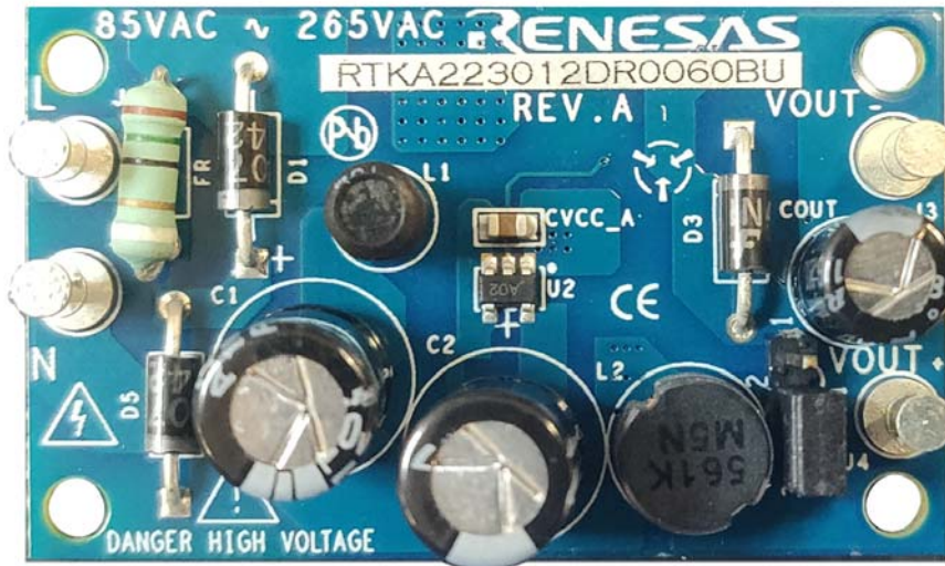
Figure 4. RTKA223012DR0060BU Evaluation Board (Top)
