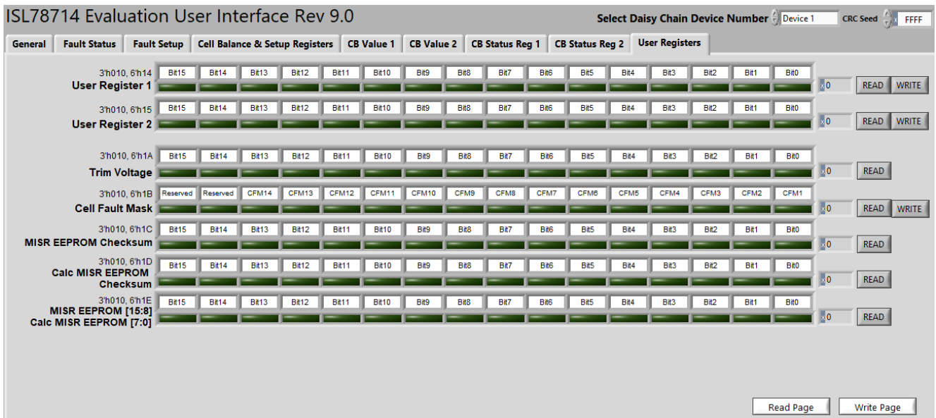
Figure 20. User Registers and EEPROM Tab Layout
