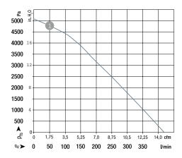
Breathing device applications demand fans with highly dynamic characteristics. A high pressure is required at the start of the breathing sequence and a low pressure at the end. In practice, that means pressure fluctuations between 400 Pa and 2000 Pa. With a centrifugal impeller, the flow quantity and delivery pressure increase with increasing speed. The high nominal speed of 40,000 rpm thus produces dynamic power output – with a compact design.
