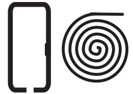
Figure 30: Loop or Trace Antenna
