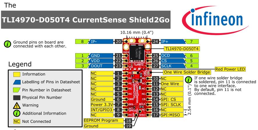
The maximum voltage on any pin is 3.6 V.
