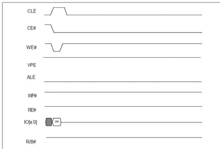
Figure 14. Waveforms for the Lock-down Command
