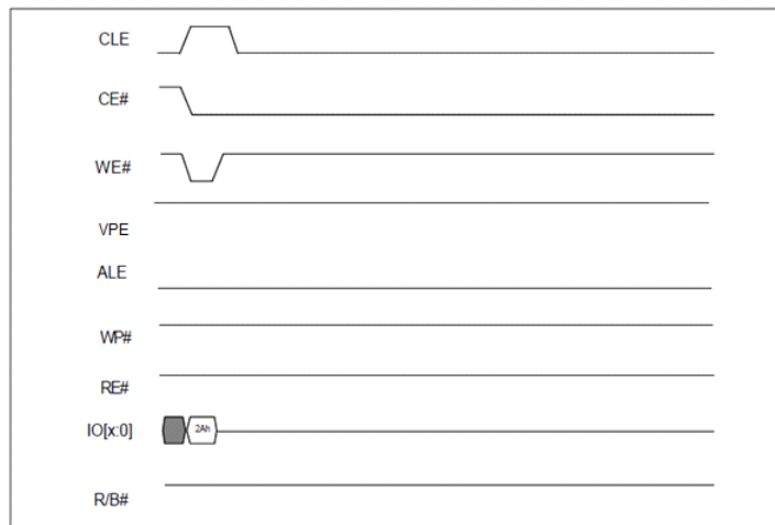
Figure 9. Waveforms for the Lock-down Command
