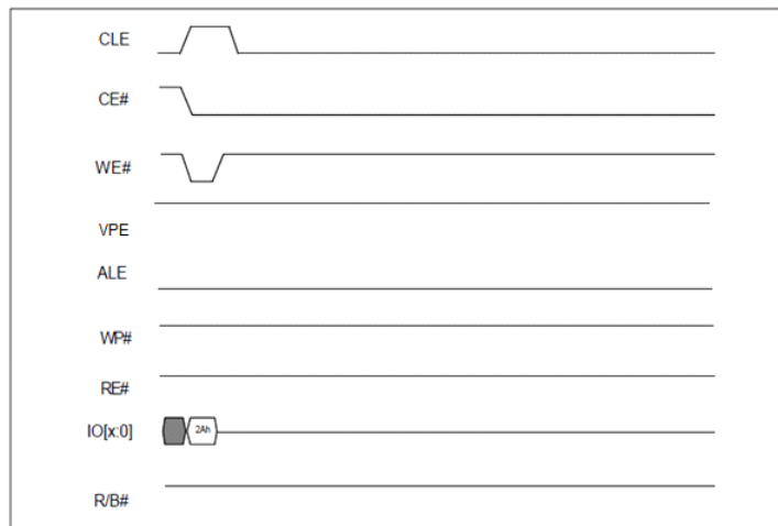
Figure 8. Waveforms for the Lock-down Command
