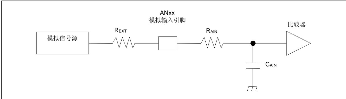
(式 1)  $t_s \geq (R_{AIN} + R_{EXT}) \times C_{AIN} \times 9$
