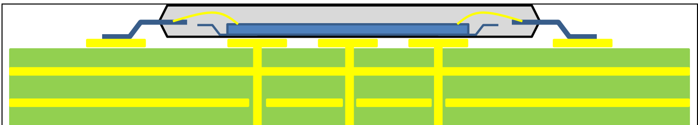
Figure 8-1: Example Thermal via Holes on PCB.
