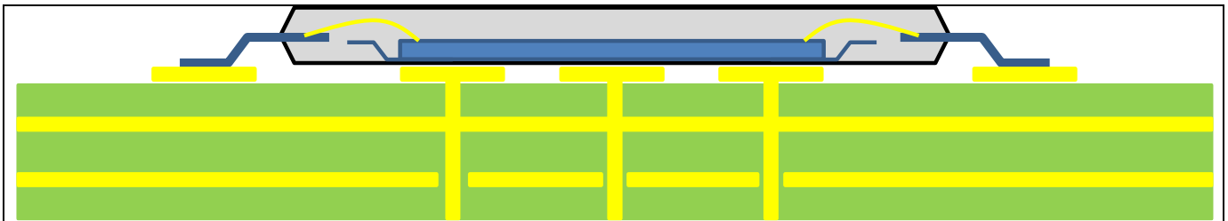
Figure 7-1: Example Thermal Via Holes on PCB.
