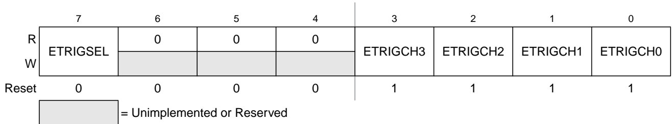
Figure 4-4. ATD Control Register 1 (ATDCTL1)
