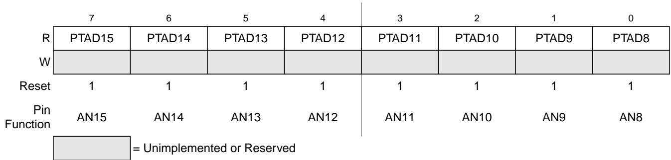
Figure 4-16. Port Data Register 0 (PORTAD0)
