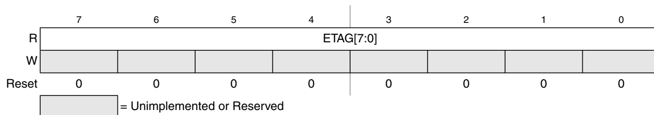
Figure 27-19. EEE Tag Counter Low Register (ETAGLO)
