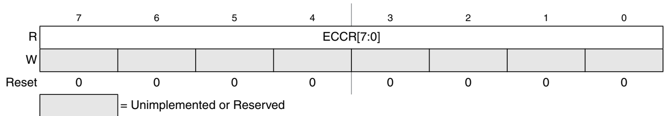
Figure 27-21. Flash ECC Error Results Low Register (FECCRLO)
