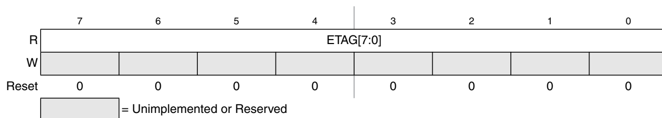
Figure 25-19. EEE Tag Counter Low Register (ETAGLO)
