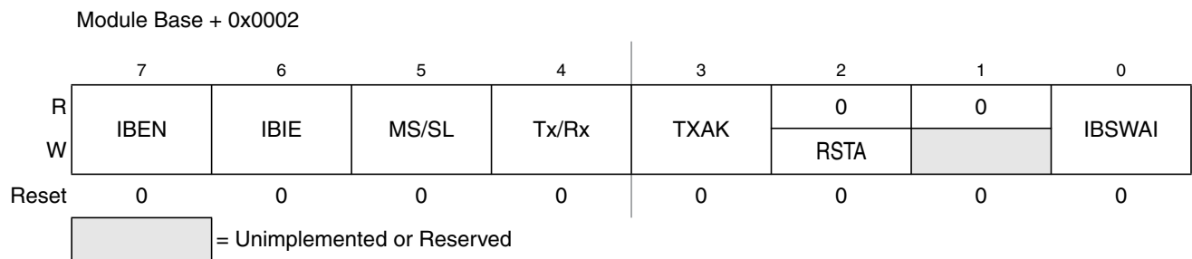
Figure 15-6. IIC Bus Control Register (IBCR)
