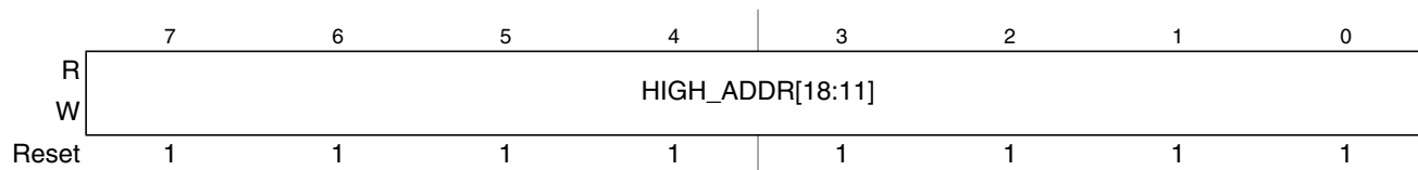
Figure 4-12. MPU Descriptor Register 4 (MPUDESC4)
