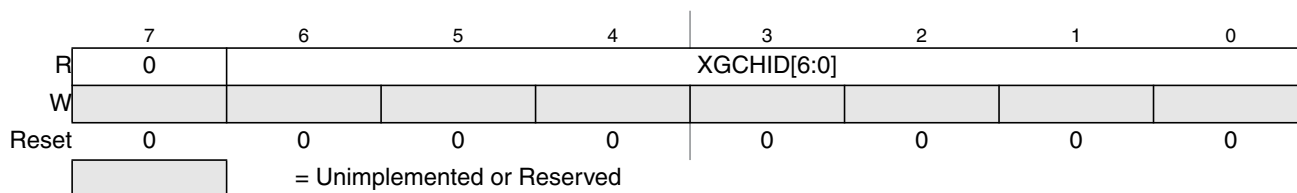
Figure 10-4. XGATE Channel ID Register (XGCHID)
